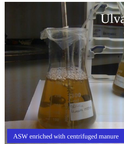
1&2: Artificial seawater (35ppt salinity) enriched with pig manure 3&4: ASW enriched with centrifuged pig manure (13500rpm) 5: ASW enriched with \text{NH}_4 6: ASW enriched with \text{NO}_3 (F/2)
