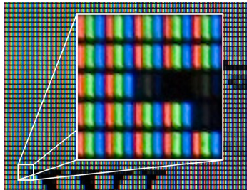
Figure 5: A close up photo of a liquid crystal display (LCD) panel. As can be seen, it is built up from a regular pattern of red, green and blue elements (sub-pixels).
