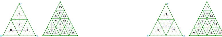
Fig. 2. A comparison of the subdivision schemes used by Gruen et al. (left), Vulkan ® and DirectX ® (right) at equivalent levels (i.e., N = 2, 4 and n = 1, 2 respectively). Note in particular the indexing order and the rounding pattern at the edges and corners, here shown with red arrows.
