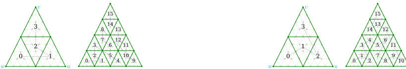
Fig. 2. A comparison of the subdivision schemes used by Gruen et al. (left), Vulkan ® and DirectX ® (right) at equivalent levels (i.e., N = 2, 4 and n = 1, 2 respectively). Note in particular the indexing order and the rounding pattern at the edges and corners, here shown with red arrows.
