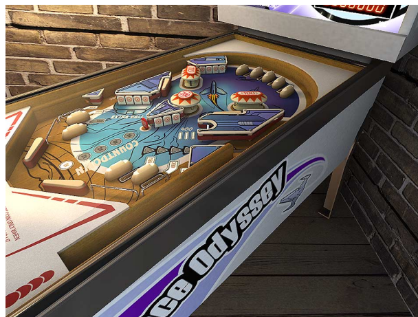
Fig. 12. This image was rendered using OpenGL ES 2.0, and 14 different vertex and pixel shader programs were used. Antialiasing using four samples per pixel was used for higher quality. (Image appears courtesy of AMD.)
