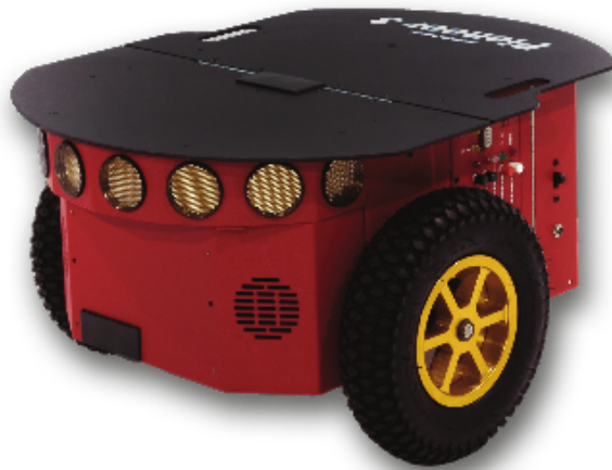
Figure 8.12: Pioneer 3-DX, an all-purpose base, used for research and applications
