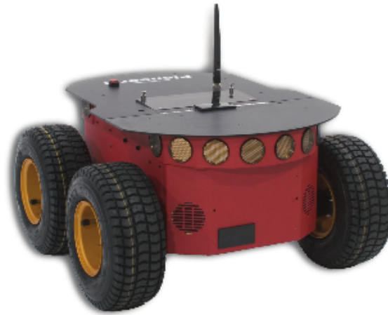
Figure 8.8: Pioneer 3-AT, a ready-to-use all terrain base
