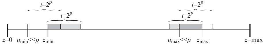
Figure 7.3: A problem with the inexpensive variant of depth offset compression is illustrated here. Since z_{\min} is truncated to u_{\min} and z_{\max} is truncated to u_{\max} , the full range of t = 2^p cannot be exploited for encoding offsets. In this figure, only the dark gray regions can actually be used. With the more expensive technique, all values in the light and dark gray regions could be encoded with offsets.
