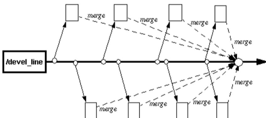
Figure 2: Big-bang integration at the end (undesirable).
