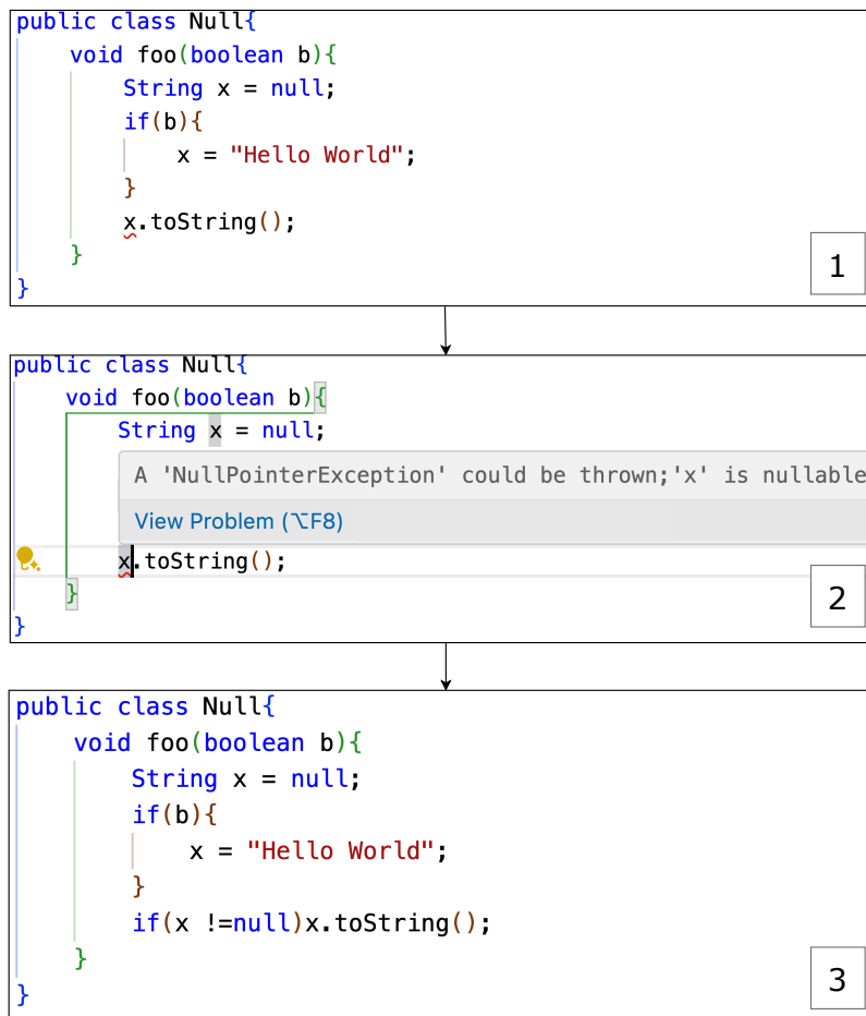
Figure 11: Bug detection and quick fix in VISUAL STUDIO CODE using INTRAJ. 1. The NullPointerException is detected by INTRAJ (squiggly line under x ) with a quick fix available (💡). 2. The user can hover over the warning to see an explanation of the issue. 3. The user can click on the quick fix icon (💡) to apply the fix.
