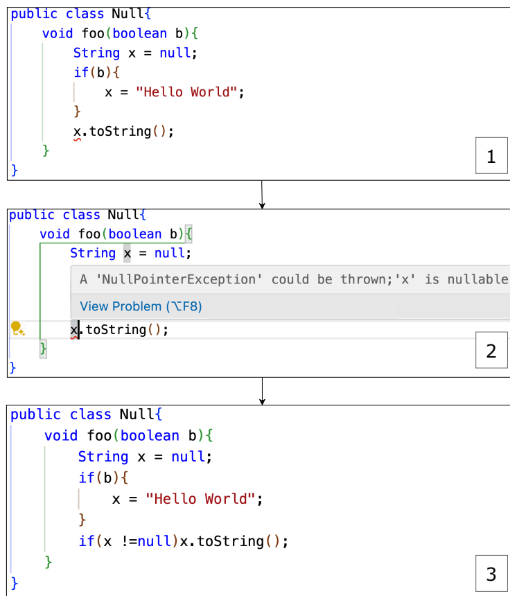
Figure 17: Bug detection and quick-fix in VISUAL STUDIO CODE using INTRAJ. 1. The NullPointerException is detected by INTRAJ (squiggly line under x ) with a quick-fix available (💡). 2. The user can hover over the warning to see an explanation of the issue. 3. The user can click on the quick-fix icon (💡) to apply the fix.
