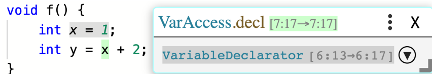
Figure 5: Example of a reference result. The decl property of the variable x has been probed, resulting in a reference to a VariableDeclarator node. The user hovers the result, causing the corresponding span in the source code ( x = 1 ) to be highlighted in gray.
