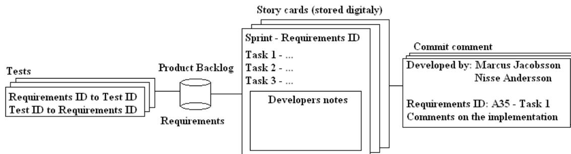
Figure 12 – A way to add test tracing
