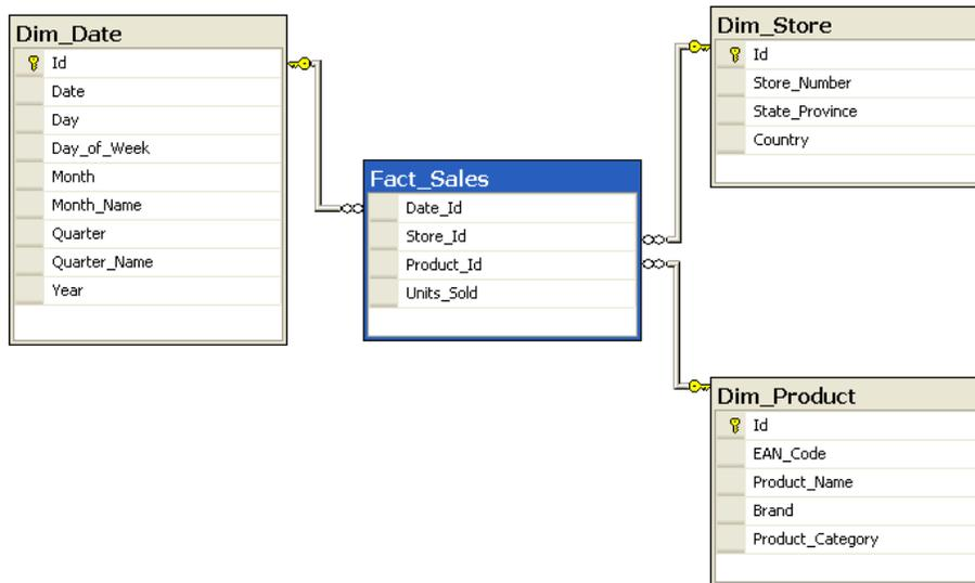
Figure 9 – An example of a star schema [22]
