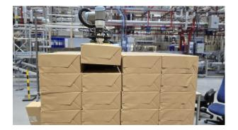
How does it work? The solution to this problem is a collaborative robot with suction cups and a depth-camera attached to the robot end-effector. The robot will then use an open source AI detection and segmentation model to detect a box and then use the suction cups to move it to the conveyor belt.
