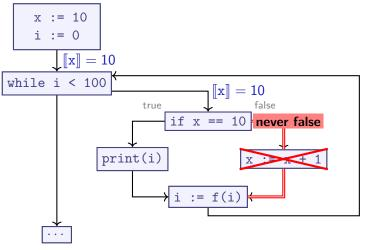
"Tight Composition": Run analyses *together*: Constant Propagation / Folding & Dead Path Elimination
