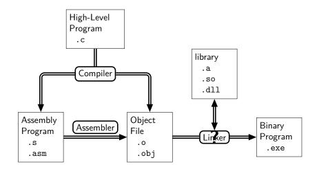
Binary program is machine code, can be run by CPU
