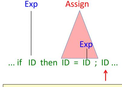
LL(1): decides to build Assign after seeing the first token of its subtree. The tree is built top down.
