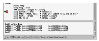
In the above image you can see that the previous base pointer was zero, the return address is 0x4000bb, and the first parameter is 0x86.
