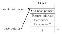
Now we can go ahead and push local variables on the stack, and use RBP to address those local variables. For example, the first local variable would have the address -8(%rbp), because it is right above RBP on the stack which means it has a lower address and its size is 8 bytes, hence the -8.
