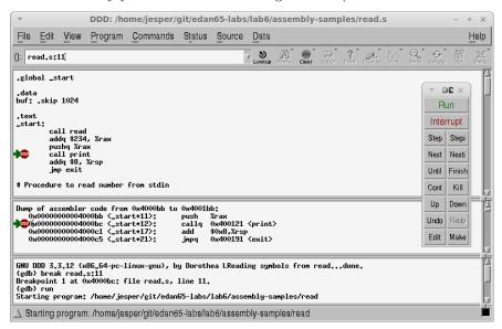
If the source code is missing (as indicated by a mostly blank window), it means that you forgot to use the --gstabs option with as.
