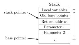
All that remains now is to jump back to the return address and to pop parameters off the stack. We can use the RET instruction, which pops the return address off the top of the stack then jumps to that address. The parameters are still left on the stack after returning to the caller though, so the caller must ensure that they are removed:
