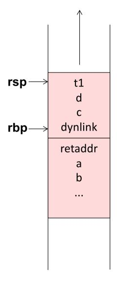
Understand how an activation stack works, with frame pointer, stack pointer, and dynamic link.
