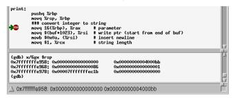
In the above image you can see that the previous base pointer was zero, the return address is 0x4000bb, and the first parameter is 0x86.
