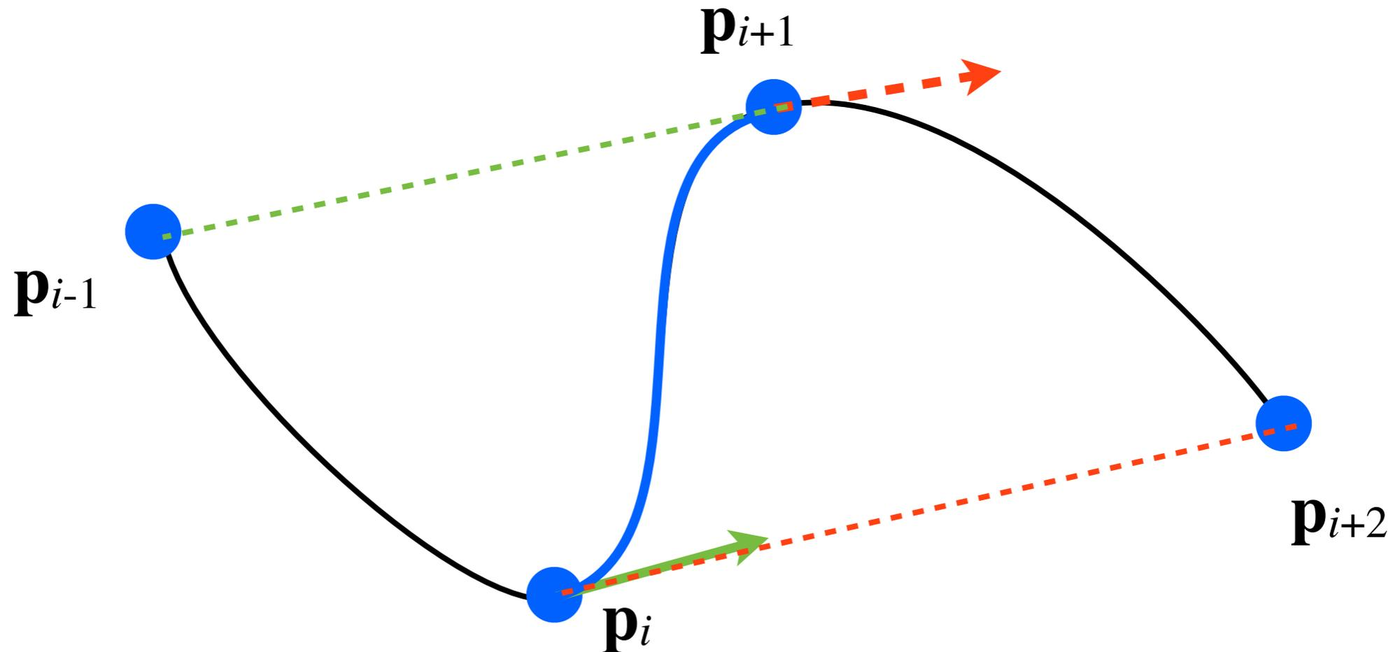
Use **four points** to specify **cubic curve segment**. No need to manually specify tangents. Tangents approximated by:
