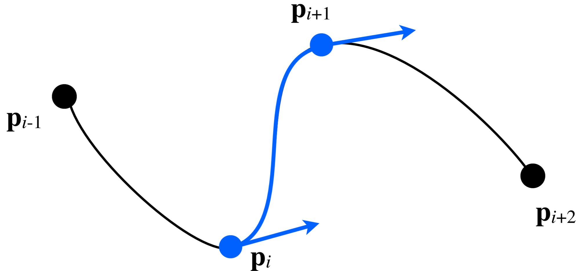
Use two points and two tangents to specify **cubic** curve segment
