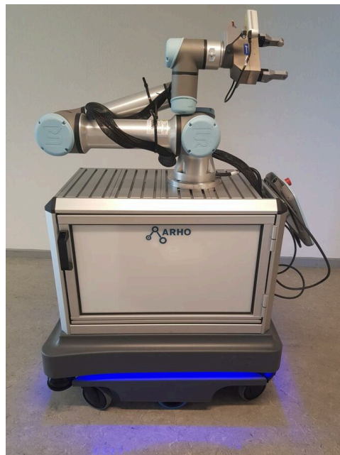
Figure 3: Robot used for the purpose of the system design and operation. Universal Robot arm UR5e mounted on a MiR200.
