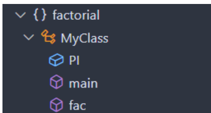
Fig. 6: The document outline for a Java program when using ExtendJ and JastAdd Bridge.
