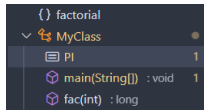
Fig. 7: The document outline for a Java program when using the Red Hat language server.
