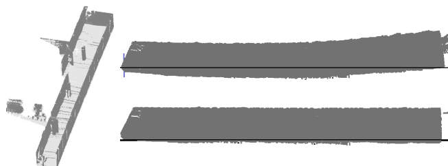
Fig. 1. Left: Map, top view. Right, top: The unconstrained 3D mapping shows a banana-shaped form. Right, bottom: The horizontal justification and the constrained mapping lead to qualitatively correct maps.
