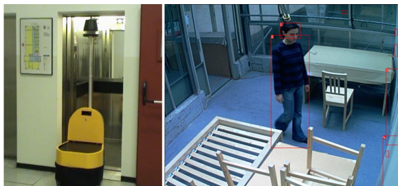
Fig. 2. (Left) Staffetta entering the elevator; (Right) User tracking through cameras.
