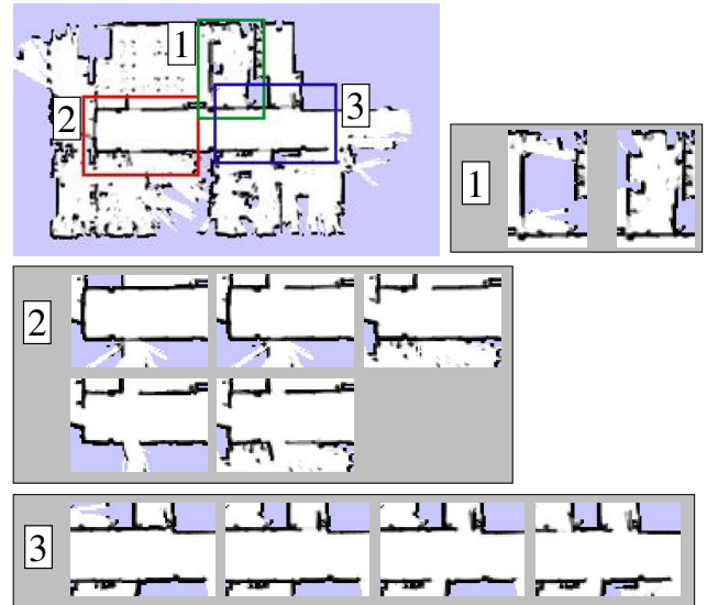
Figure 2: A patch-map representing the different configurations learned for the individual sub-maps in a typical office environment.
