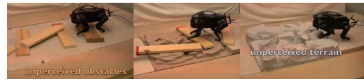
Fig. 10. The LittleDog robot and various setups to test the robustness of the controller towards non-perceived obstacles and terrains. Please see the video supplement.
