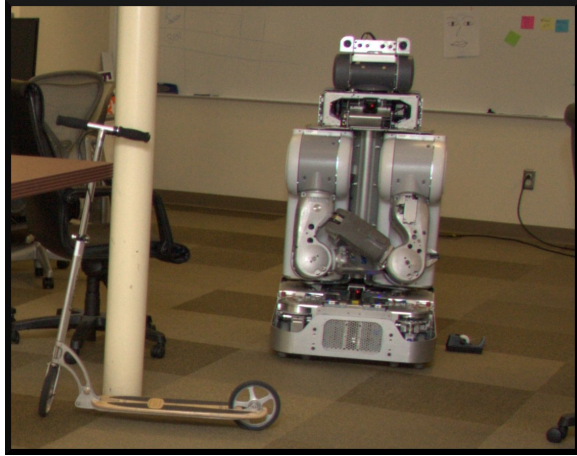
Fig. 7. The robot avoiding a tape dispenser and a scooter in an obstacle slalom course.
