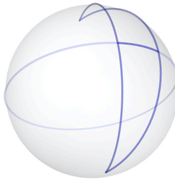
Figure 5: A spherical digon, or lune. The two antipodal points are connected by two arcs of length \pi . The area of the lune equals twice the length of the arc it spans on the great circle orthogonal to both arcs.
