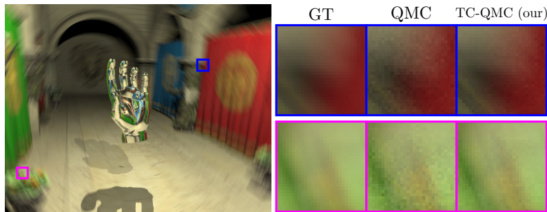
Figure 8: SPONZA+HAND equal-time comparison. QMC obtains a PSNR of 38.4 dB in 10.0 s (32 shading samples per pixel), while TC-QMC (our) obtains 41.3 dB in 9.9 s (49.3 shading samples on average). The zoom-ins on the pillar/drape and on the plant highlight the low level of noise achieved by time-continuous visibility. The HAND model, which is static in camera space, is detected by our algorithm to be static, causing it to be sampled stochastically instead of time-continuously.
