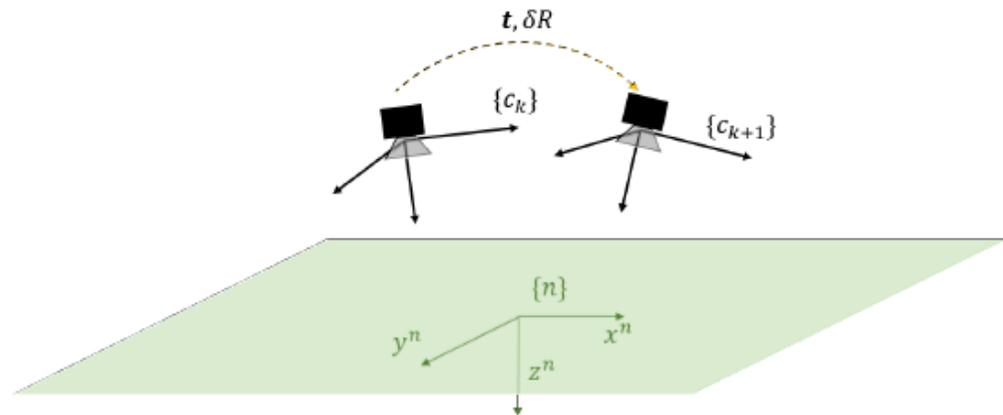
**Figure 3.10:** With epipolar geometry it is possible to find a dimensionless translation  $t$  and the relative rotation,  $\delta R$ , from time  $t_k$  to  $t_{k+1}$  without any prior information about the structure.
