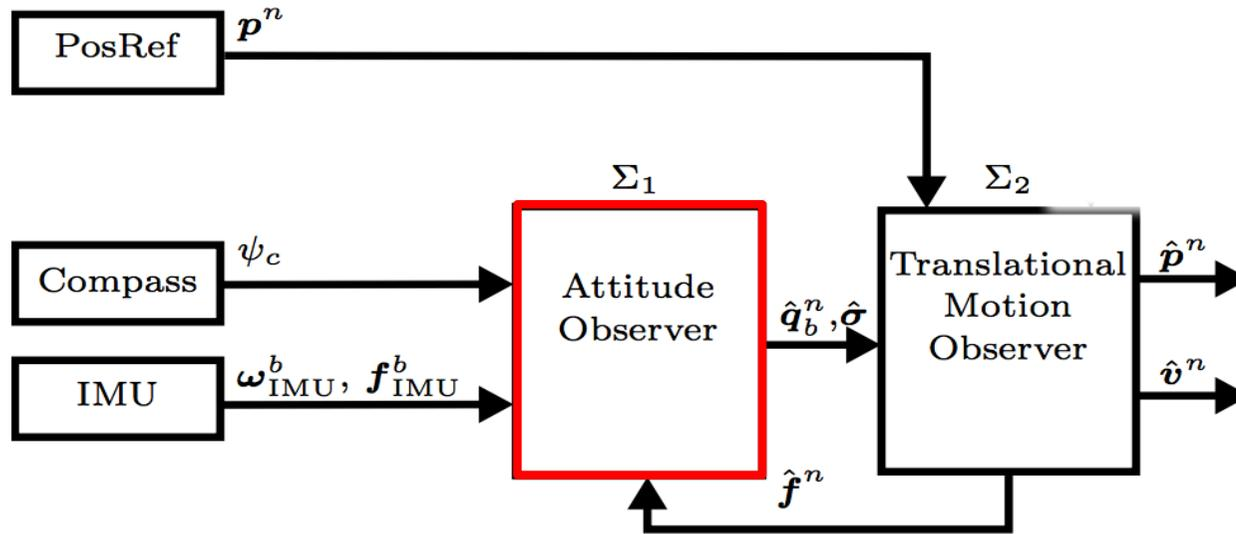
Feedback interconnection where the specific force  $f^n$  is estimated. Important for highly accelerated vehicles.
