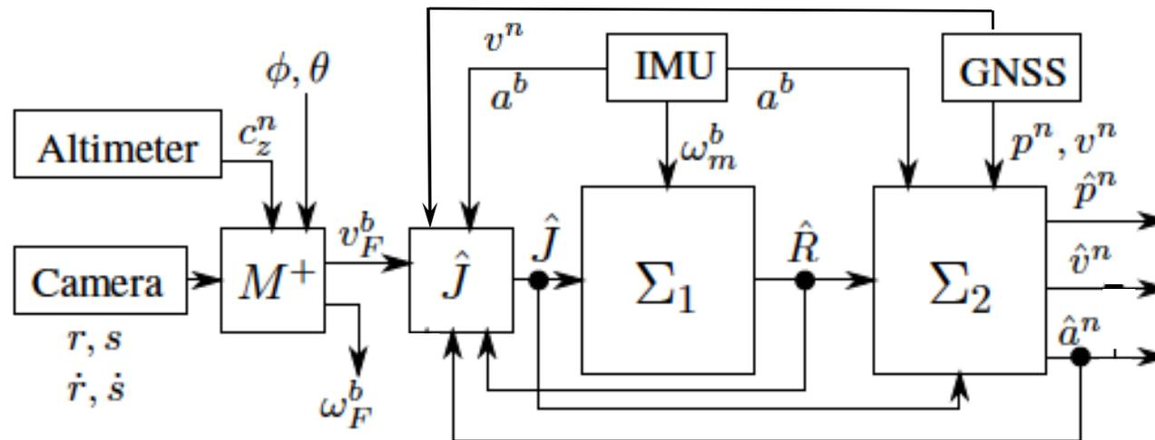
The origin of the feedback interconnection  $\Sigma_1$ – $\Sigma_2$  (feedback from estimated NED acceleration  $a^n$ ) is **GES** if the roll and pitch angles in the M-matrix are auxiliary signals typically obtained by:
