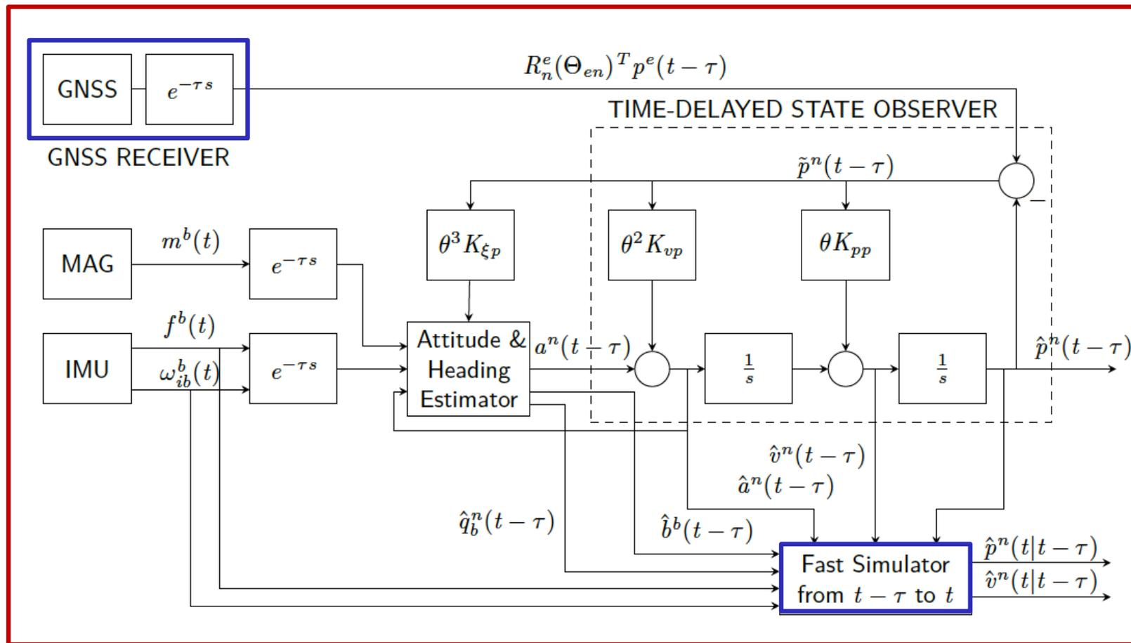
A fast simulator (predictor) is used to predict the current position and velocity.
