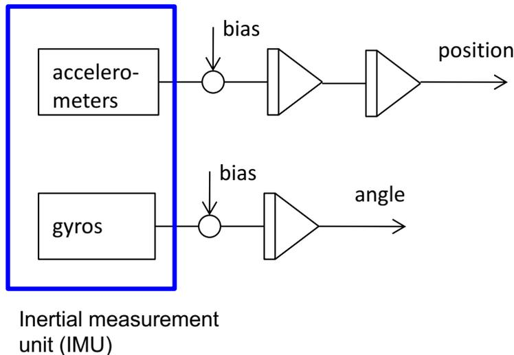
The integrated signals will drift. Hence, the system must be **aided** by GNSS, hydroacoustic positioning reference (HPR) systems or other reference systems.
