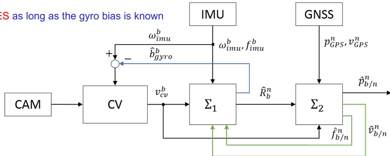
Do not need roll angle  $\varphi$  and pitch angle  $\theta$  nor attitude  $h$  to compute the transformation matrix  $CV$
