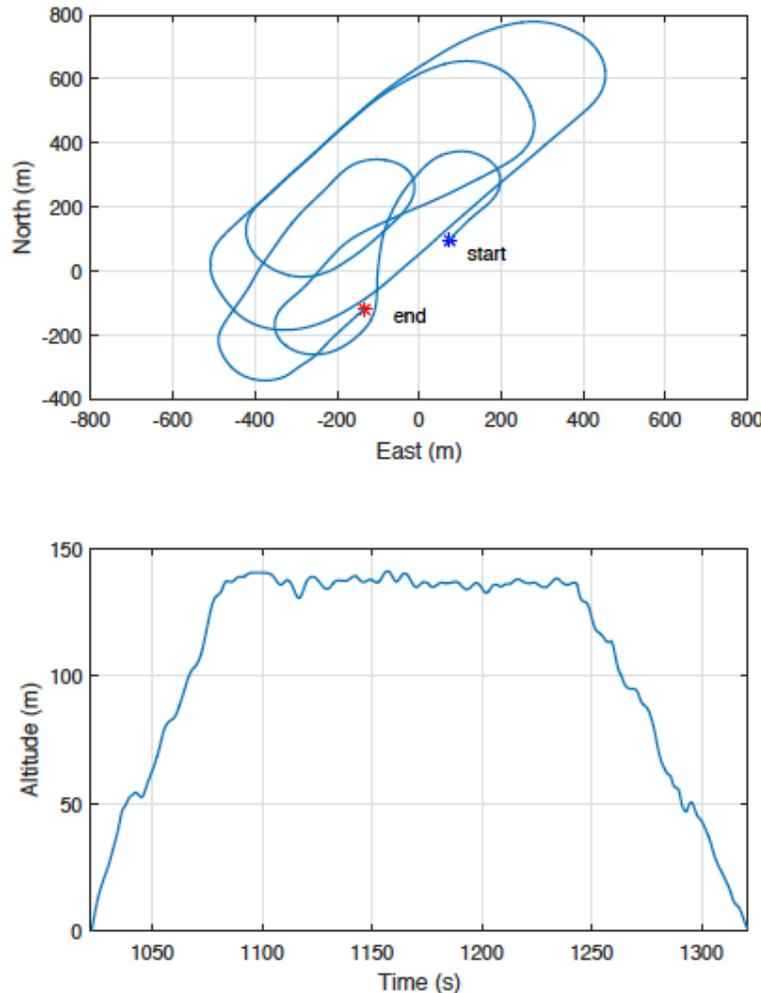
Fig. 5. Position on the N-E plane and altitude, as output by the EKF, used as reference. The blue and red stars indicate the start and end of the data set, respectively.
