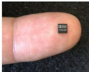
**Micro-electro-mechanical system (MEMS)** accelerometer technology capable of tracking vibrations in industrial equipment at frequencies as high as 22 kHz. Analog Devices (2008)
