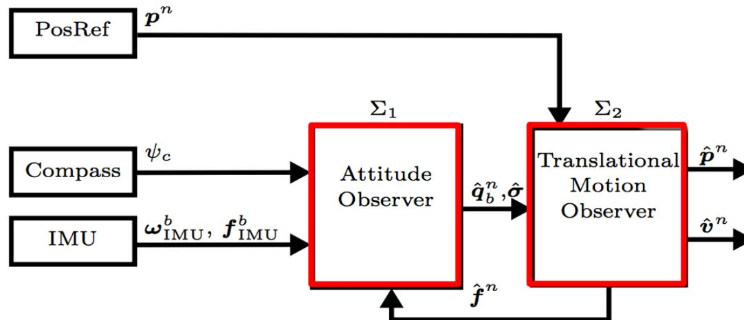
**Dead reckoning** is referred to as the case when the PosRef systems fail and position and linear velocity are predicted using the observers without PosRef updates.
