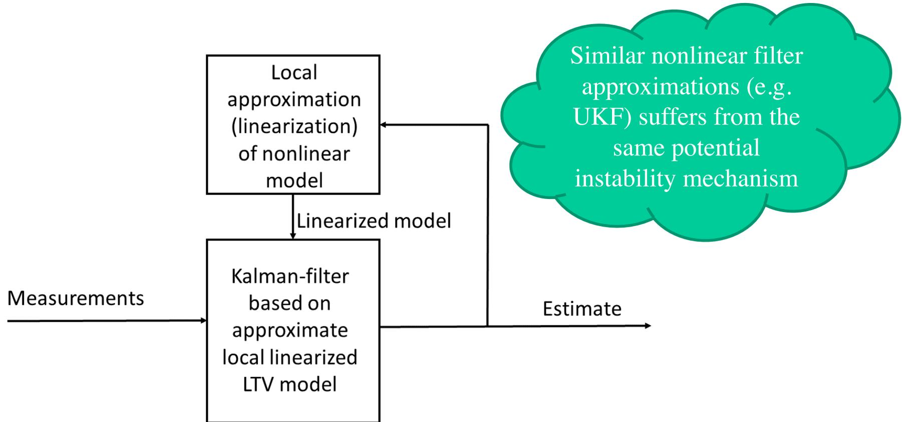
Using the state estimate for linearization creates a **feedback loop** that can **destabilize the EKF** if the state estimate is not sufficiently accurate.
