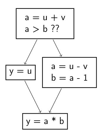
Basic block: sequence of instructions with no label or branch CFG: directed graph with basic blocks as nodes and branches as edges
