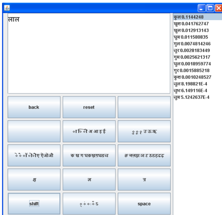
Figure 4.3: The Hindi GUI after shift has been pressed. The compound letters can be seen in the fourth row from the top.
