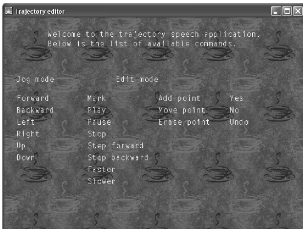
Figure 1: SAPI 5.1 speech interface application front end with a list of available command words.
