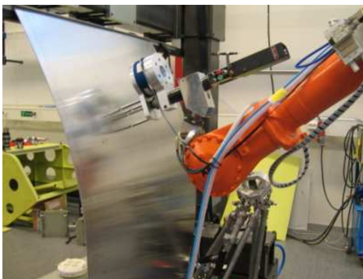
Figure 4.9 Set-up for testing of drilling in flexible airframe skin panels according to task-level program of Fig. 4.8.
