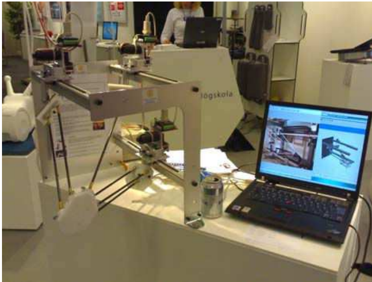
Figure 5.2 Table-sized Gantry-Tau prototype shown at the Scandinavian Technical Fair (Stockholm, 3-6 October, 2006). End effector, linear tracks, and gearboxes manufactured inhouse. Drive systems from the Faulhaber Group [6]. Robot controlled from the Visual Components 3DCreate tool (laptop).
