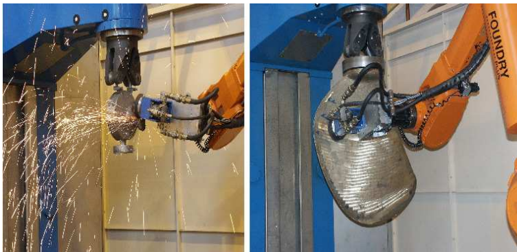
Figure 3.11 Stub-grinding (left) and finishing on a propeller blade (right).
