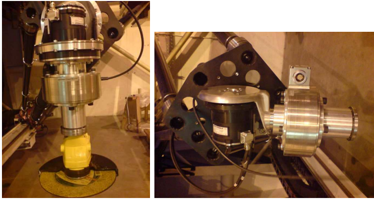
Figure 5.5 The 2-DOF serial wrist with two lightweight actuators including high-power HDD-motors mounted on the (black) “wrist frame plate”. A wrist-mounted force/torque sensor (ATI Omega160) is used for lead-through programming and contact force controlled cutting/grinding.
