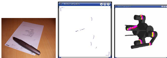
Figure 8.5 Foundry workpiece experiment. In upper picture the pen with the CAD model of the foundry workpiece printed on the paper enabling the Anoto technology and the pen strokes specify the cuts to be made. In the lower part, the imported pen strokes (left) and the surface mapping on workpiece 3D image.
