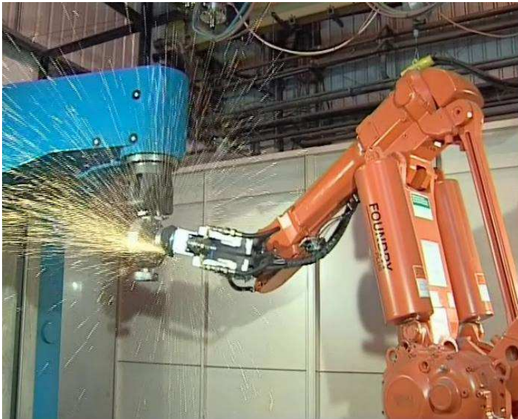
Figure 3.6 Force controlled stub grinding using an ABB Irb6400 industrial robot with an extended ABB S4CPlus control system.
