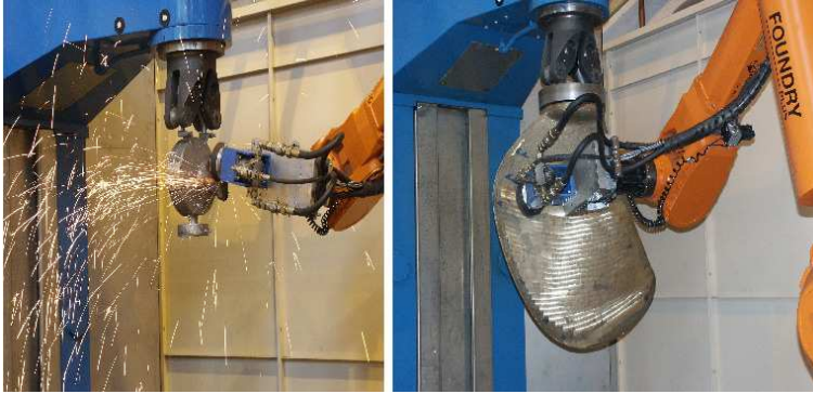
Figure 3.10 Stub-grinding (left) and finishing on a propeller blade (right).
