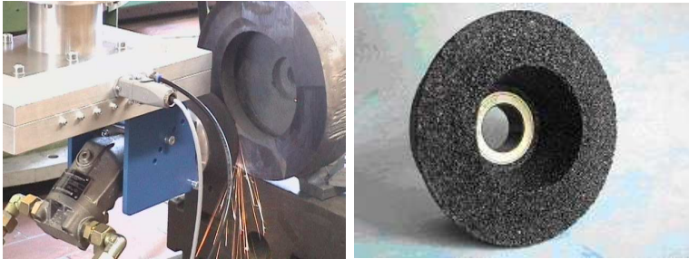
Figure 3.7 The developed compliant grinding tool (left) and cup stone (right) for stub-grinding application.
