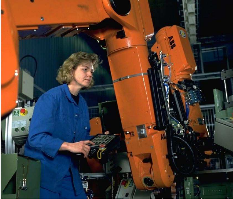
Figure 6.4 Robot operator/programmer at Volvo, using a hand-held terminal for online changes. (With permission from Volvo and ABB).
