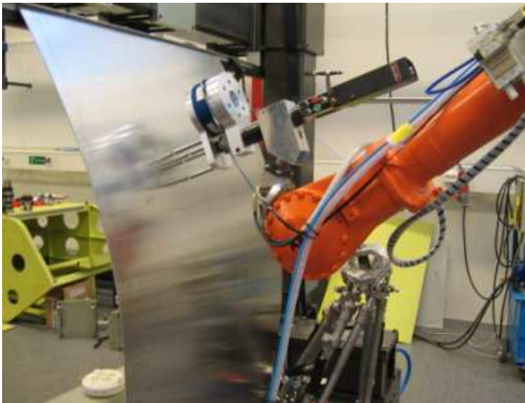
Figure 4.7 Set-up for testing of drilling in flexible airframe skin panels according to task-level program of Fig. 4.6.
