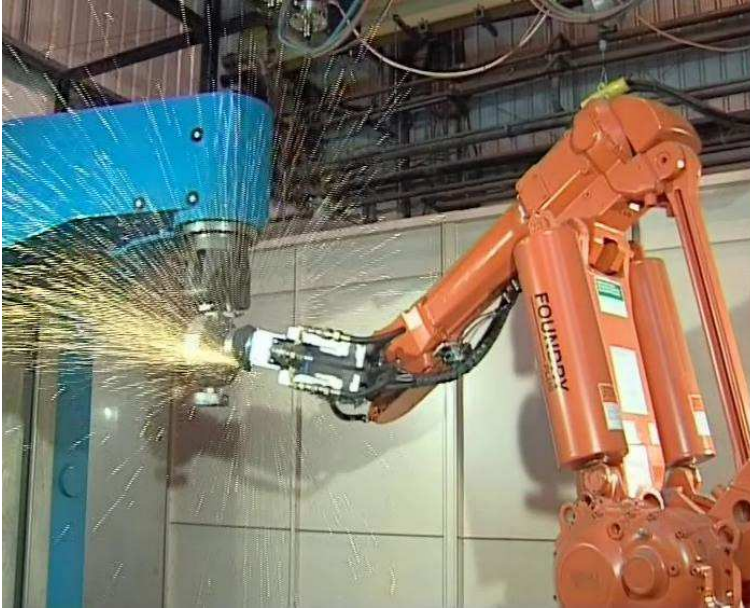
Figure 3.5 force-controlled stub grinding, as carried out by an ABB IRB 6400 industrial robot with an extended ABB S4CPlus control system.
