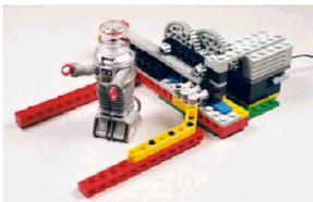
Robot Gripper Using Gear Rack
