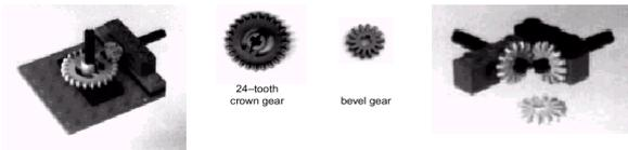
The 8-tooth gear, in conjunction with the 24-tooth **crown gear**, is used to **change the axis of rotation** in a gear train. In this instance, the configuration provides for a **vertical shaft output**. Horizontal output also possible.
