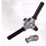
The "**toggle joint**" can be used to lock two axles at a variety of odd angles. The short axle running through the two toggle joints is equipped with stop bushes on either end to hold the joint together.
