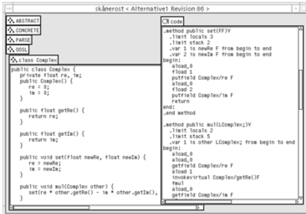
Figure 3. Source code (left) and the corresponding compiled bytecode (right).
