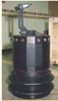
Figure 2.6: The robot at NRL, equipped with laser light emitter and tuned camera for gesture recognition
