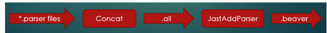
Figure 1. How JastAddParser is used in ExtendJ. Several .parser files are concatenated to an .all file which is fed to JastAddParser, producing a .beaver file for later processing by Beaver.
