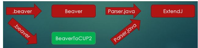
Figure 2. The way additional parser support was implemented. Instead of sending the .beaver file produced by JastAddParser to Beaver, it is sent to the grammar translator, BeaverToCUP2, producing a CUP2 parser that can be used with ExtendJ.
