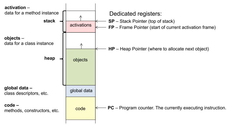
The figure shows typical use for statically loaded languages like Simula and C++. For languages with dynamic loading (like Java, Smalltalk, ...), class descriptors and code are placed on the heap, rather than in the global data and code segments.
