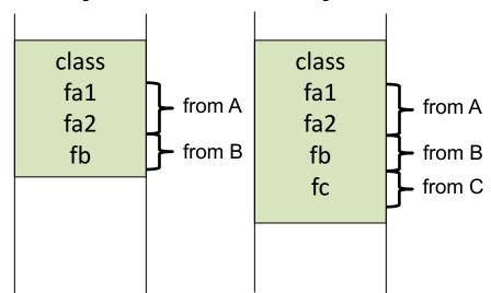
Prefixing Fields of the superclass are placed in front of local fields ("prefixing"). Each field is thus located at an offset computed at compile time, regardless of the dynamic type of the object.
