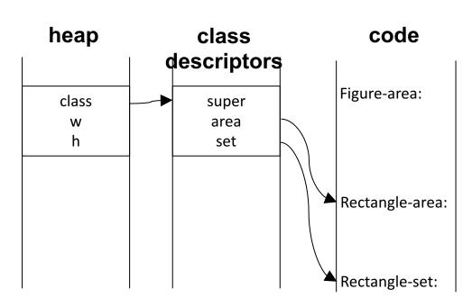
Suppose this language is implemented using virtual tables. Draw a sketch over the memory showing a Rectangle object, its class descriptor, and its code. Your sketch should include fields, class link, virtual table, and methods.
