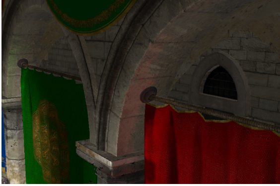
Figure 15: A closeup of colour bleed near the drapes in the scene, with a quadratic function used for the range check. Colour bleed strength was scaled to make it more apparent for the screen capture. Note the sharp cutoff of the bleed for fragments "behind" the drape.
