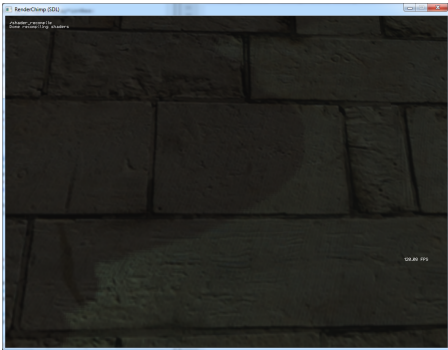
Figure 4: SFW shadow mapping with Percentage Closer Filtering applied.
