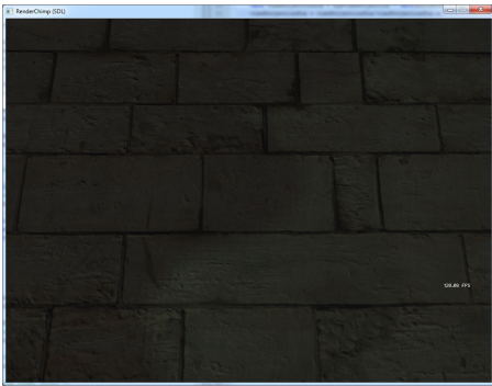
Figure 3: Conventional shadow mapping with Percentage Closer Filtering applied.
