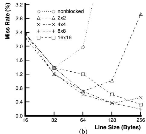
**FIGURE 5.4. The interaction between block size and cache line size. These results were measured using fully associative 32KB caches. The block dimensions are given in texels. (a) Town-vertical. (b) Guitar-horizontal.**
