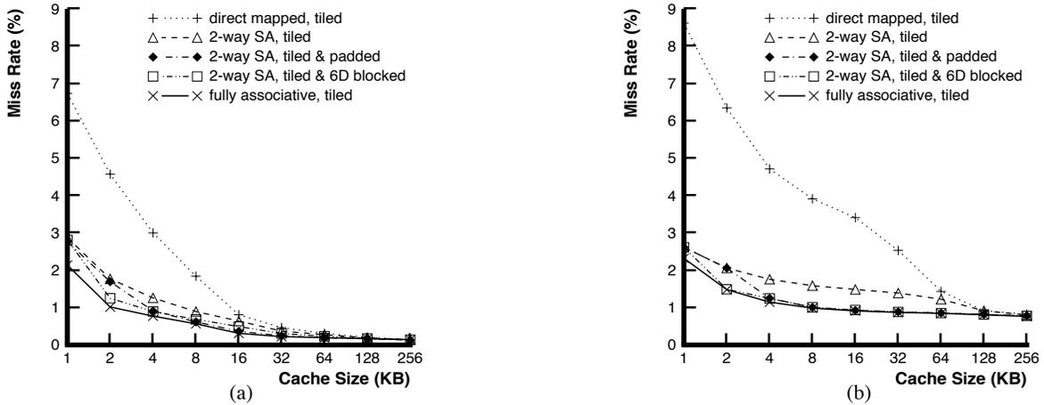
**FIGURE 6.4. Effect of tiled rasterization on conflict misses. The textures are stored in blocks of 8x8 texels and the cache line size is 128 bytes. The tiles are 8x8 pixels. The padded results use a pad of four blocks at the end of each row of texture blocks. For the 6D blocked results, we use the largest block size for the coarser blocks that is less than or equal to the cache size.**
