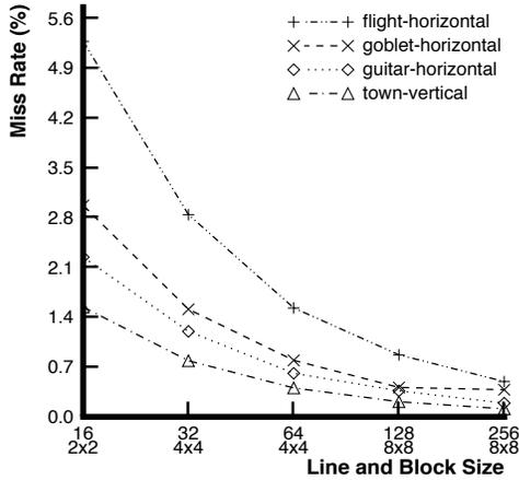
FIGURE 5.5. Effect of changes in line and block size on miss rates for all four scenes. These results were measured using fully associative 32KB caches. The block dimensions are given in texels.
