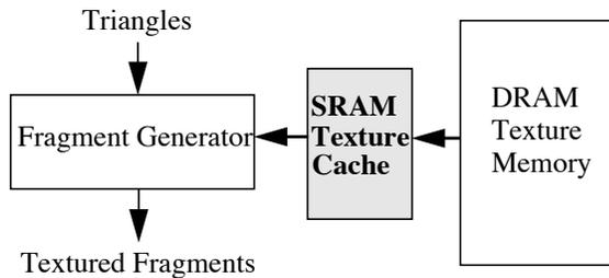
**FIGURE 2.1. Block diagram of texture mapping hardware.**
