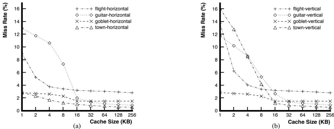
**FIGURE 5.2. Results for the base representation using fully associative caches. The line size is 32 bytes (8 texels). (a) Horizontal rasterization (row major order). (b) Vertical rasterization (column major order).**
