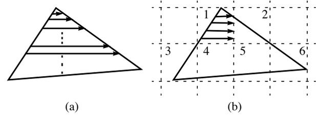
**FIGURE 6.1. (a) Illustration of nontiled horizontal rasterization, (b) Illustration of tiled rasterization. The arrows indicate the rasterization path within a tile and the numbers indicate the order in which the tiles are rasterized.**
