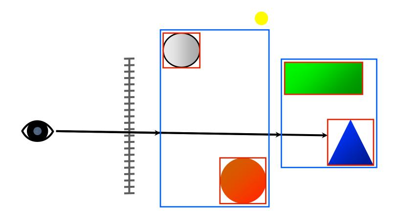
Bounding Volume Hierarchy (BVH) is most the common acceleration structure for ray tracing
