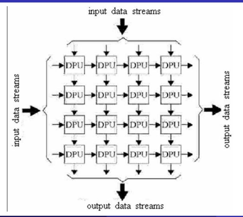
• The British Collosus code breaking machines also used the idea of systolic arrays. 10 such machines were used until the end of WWII.
