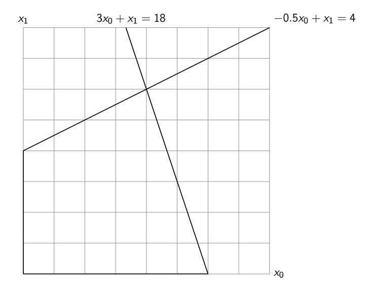
${\scriptstyle \bullet}$  Objective function and linear constraints using  $\leq$
