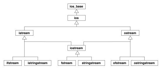
The classes ios\_base and ios contain, among other things, information about the stream state. There are, for example, functions bool good() (the state is ok) and bool eof() (end-of-file has been reached). There is also a conversion operator operator bool() that returns true if the state is good, and a bool operator!() that returns true if the state is not good. We have used these operators with input files, writing for example while (infile >> ch) and if (!infile).
