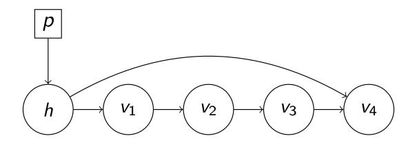
• A header node with pointers both to first and last nodes
