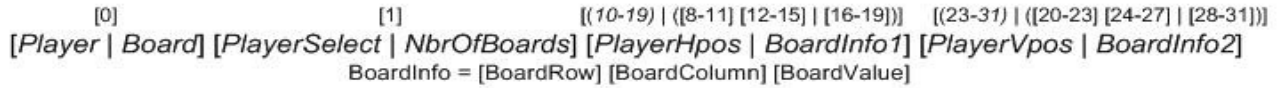
Figure 3. Transfer protocol between microblaze and graphic accelerator. First row show bit position with 0 as MSB, second row show the info contained in the bits.
