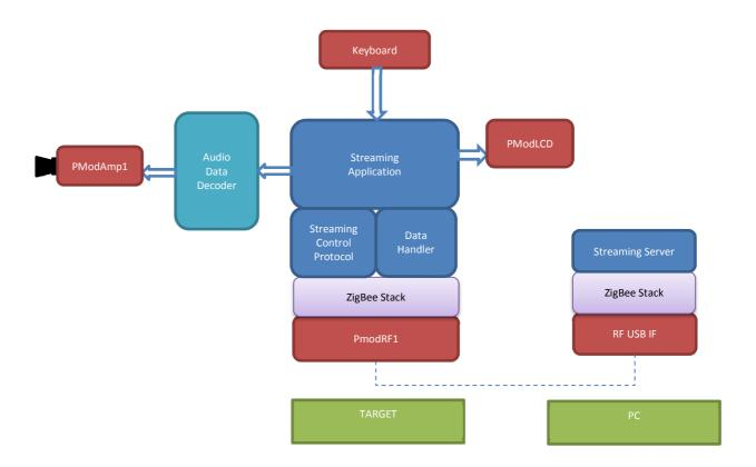
Figure 1: Block Diagram
