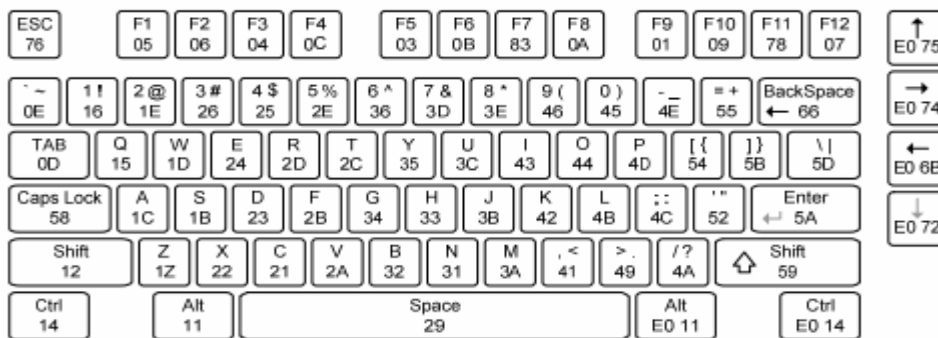
Figure 4 : PS/2 Keyboard Scan Codes
